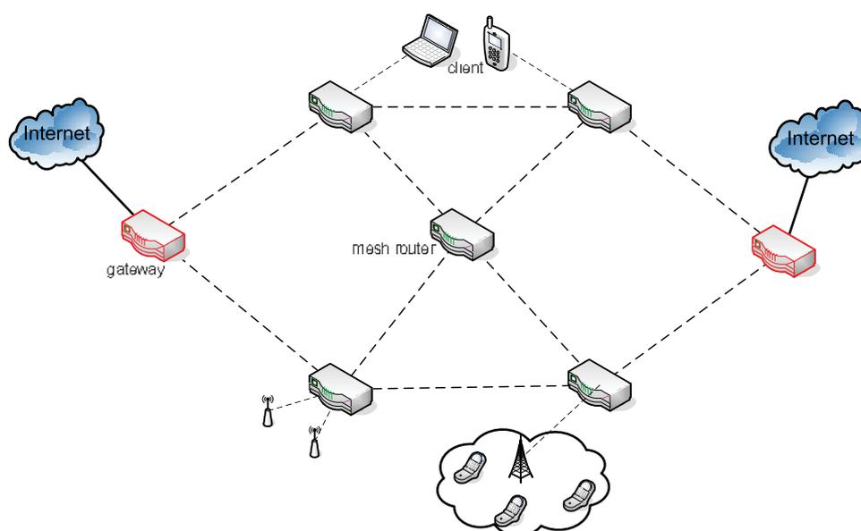
Figure 1: A typical WMN architecture.
