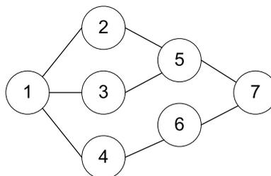
Figure 7: An illustration of equal-cost multi-path split.
